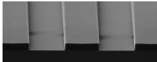
5, 10, 25  $\mu\text{m}$  features, 5  $\mu\text{m}$  thick PermiNex® 1000 coating
