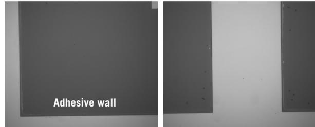
10 µm thick polymer adhesive cavity wall
