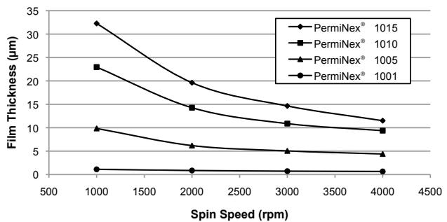
Figure 2. PermiNex 1000® Thickness vs. Spin Speed
