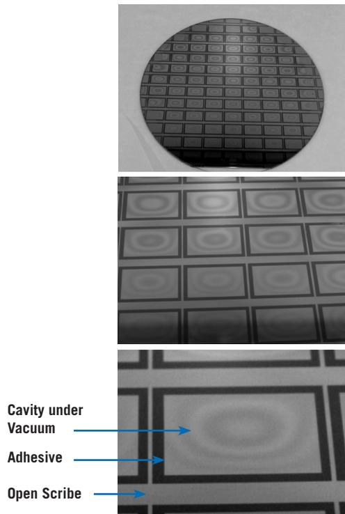
Bonded glass to silicon test cavity structure
